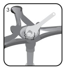
Tighten the bolt with a spanner.
