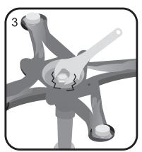
Tighten the bolt with a spanner.
